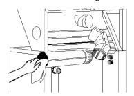
Make sure exhaust hood is not plugged with lint. Follow the instructions in this section to reinstall your vent system.
